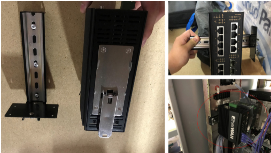
Din Rail configuration allows Din Rail devices to be mounted, which frees up more space for more devices.
