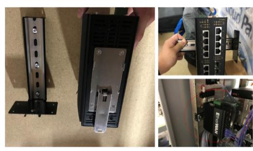
Din Rail configuration allows Din Rail devices to be mounted, which frees up more space for more devices.
